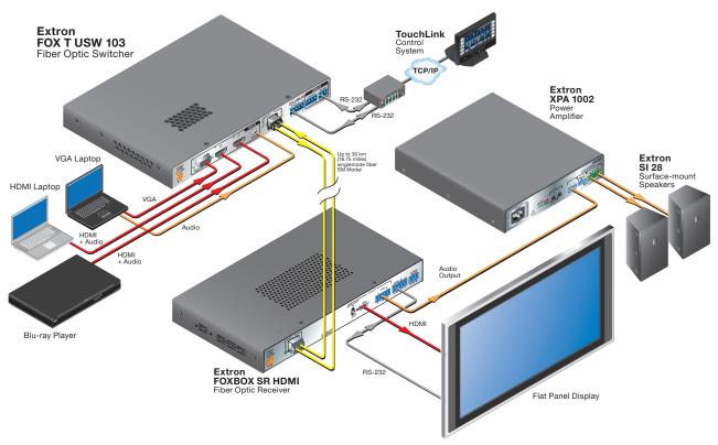
The following diagram shows a typical application of the FOX T USW 103 with three input sources, a fiber optic receiver, and control system.
